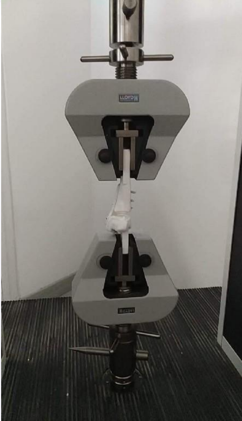
Tibia model with implanted plate on Llyod-Ametek EZ-50 Material Testing Machine
